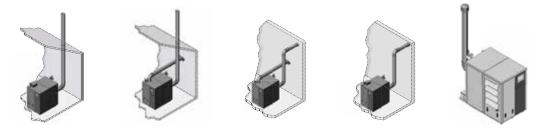
Direct or sidewall vent up to 150 feet with PVC, CPVC, Polypropylene or Stainless Steel. For detailed venting instructions review the XP PLUS water heater instruction manual at www.hotwater.com
